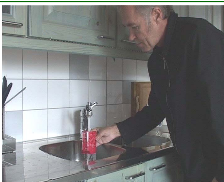
“Energy expert measuring water flow”. Photo by Markku Anttonen.
